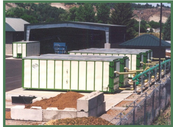
Figure 5: Static Container System
