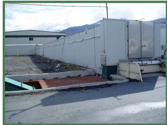
Figure 6: Wright Compost System (agitated container)
