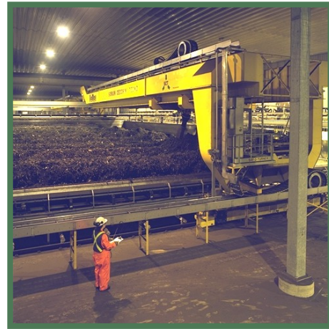
Figure 8: Agitated Bed at the Edmonton Compost Facility
