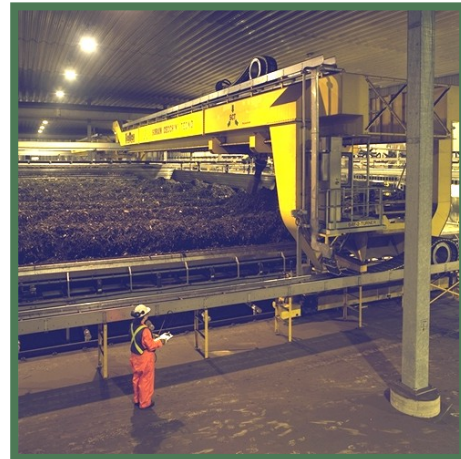
Figure 8: Agitated Bed at the Edmonton Compost Facility
