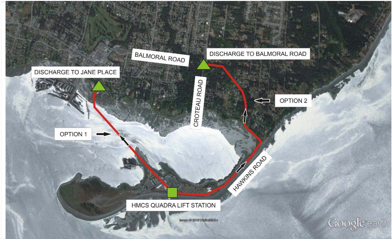
Figure 1 – Forcemain alignments Option 1 and Option 2 from HMCS Quadra to the potential point of connections.
