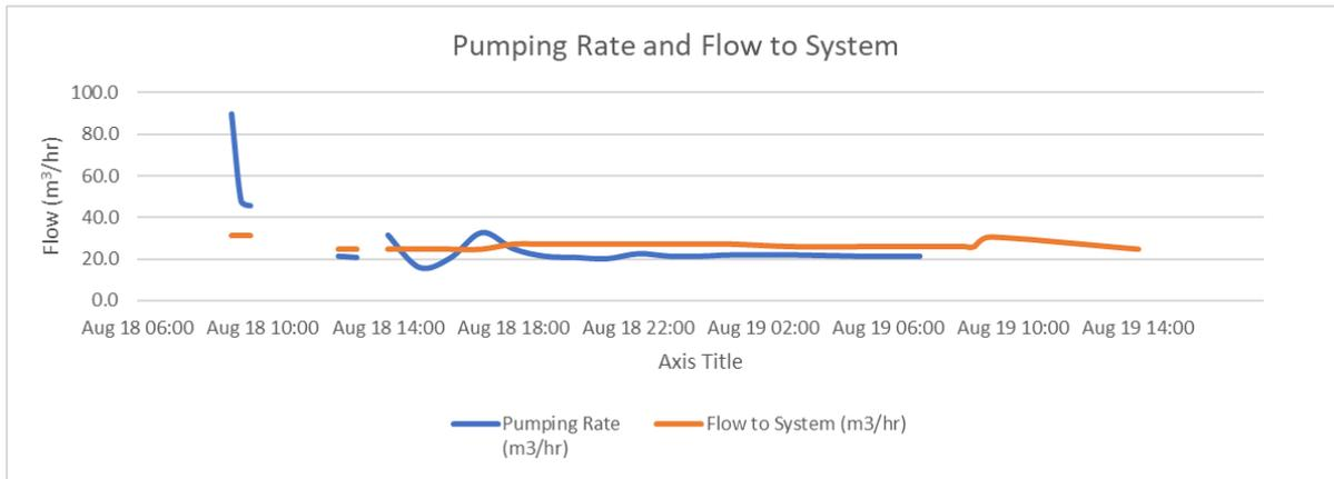
Figure 4 Pump Test Data for 18/19 August 2018
