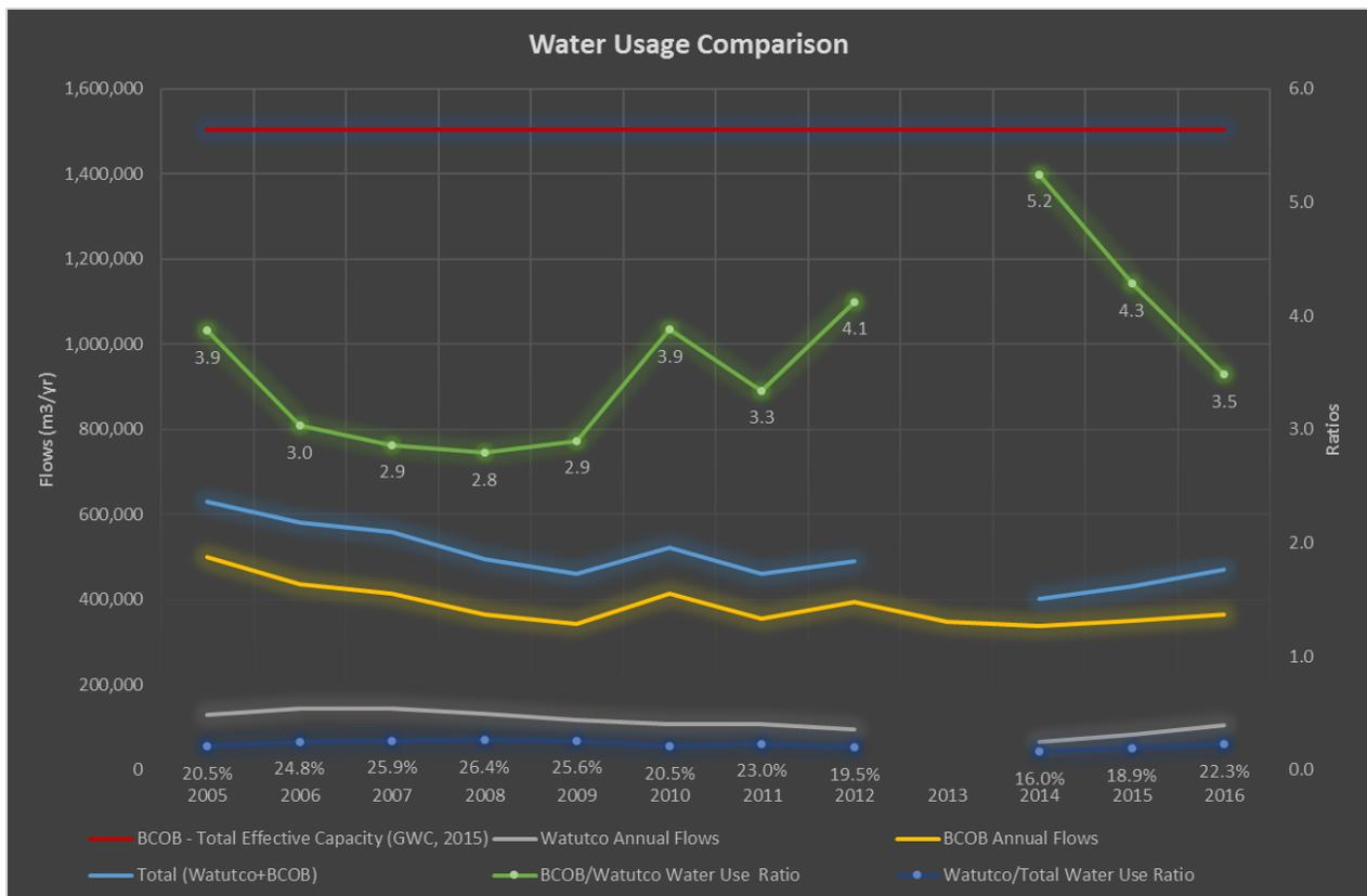
The total estimated effective capacity of the BCOB water sources in Figure 21 includes the Oyster River and ground water sources.
