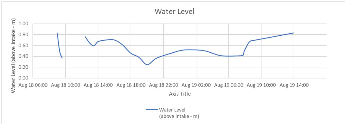
The second attempt was initiated at 12:25 pm on August 18, 2018 and ended at 7 am on August 19, 2018. During initial 4.5 hours of pumping the flow was increased from 21 m<sup>3</sup>/hr to 33 m<sup>3</sup>/hr causing the water level elevation above the intake to drop from 0.76 m to 0.24 m (refer to Figure 4). The flow rate was then reduced to approximately 22 m<sup>3</sup>/hr (refer to Figure 3) and the level stabilized between 0.4 m and 0.5 (refer to Figure 4).
