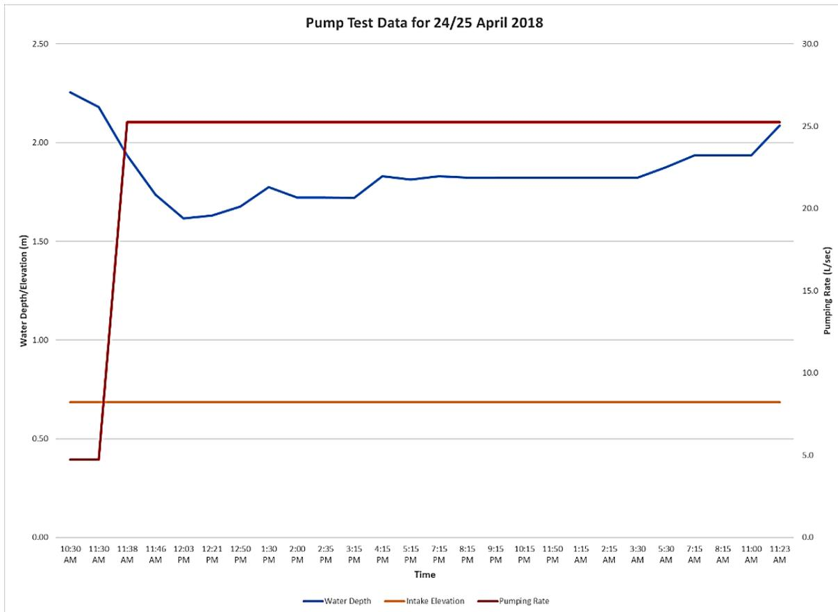
The drawdown water level in the test well stabilized after approximately three hours at an increased pumping flow rate ranging from 91 m<sup>3</sup>/hr to 157 m<sup>3</sup>/hr during Test #2 (Refer to Figure 2). The maximum observed drawdown was 1.14 m coinciding with the maximum flow rate. No water level changes were observed at the intake gallery during test duration.
