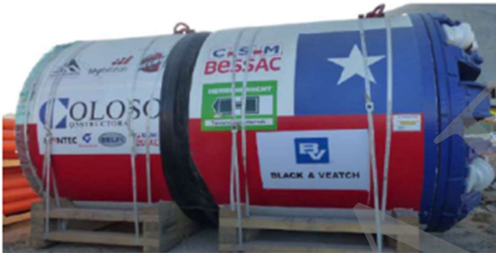
Figure 5-2: MTBM used on Escondido Water Supply Project
