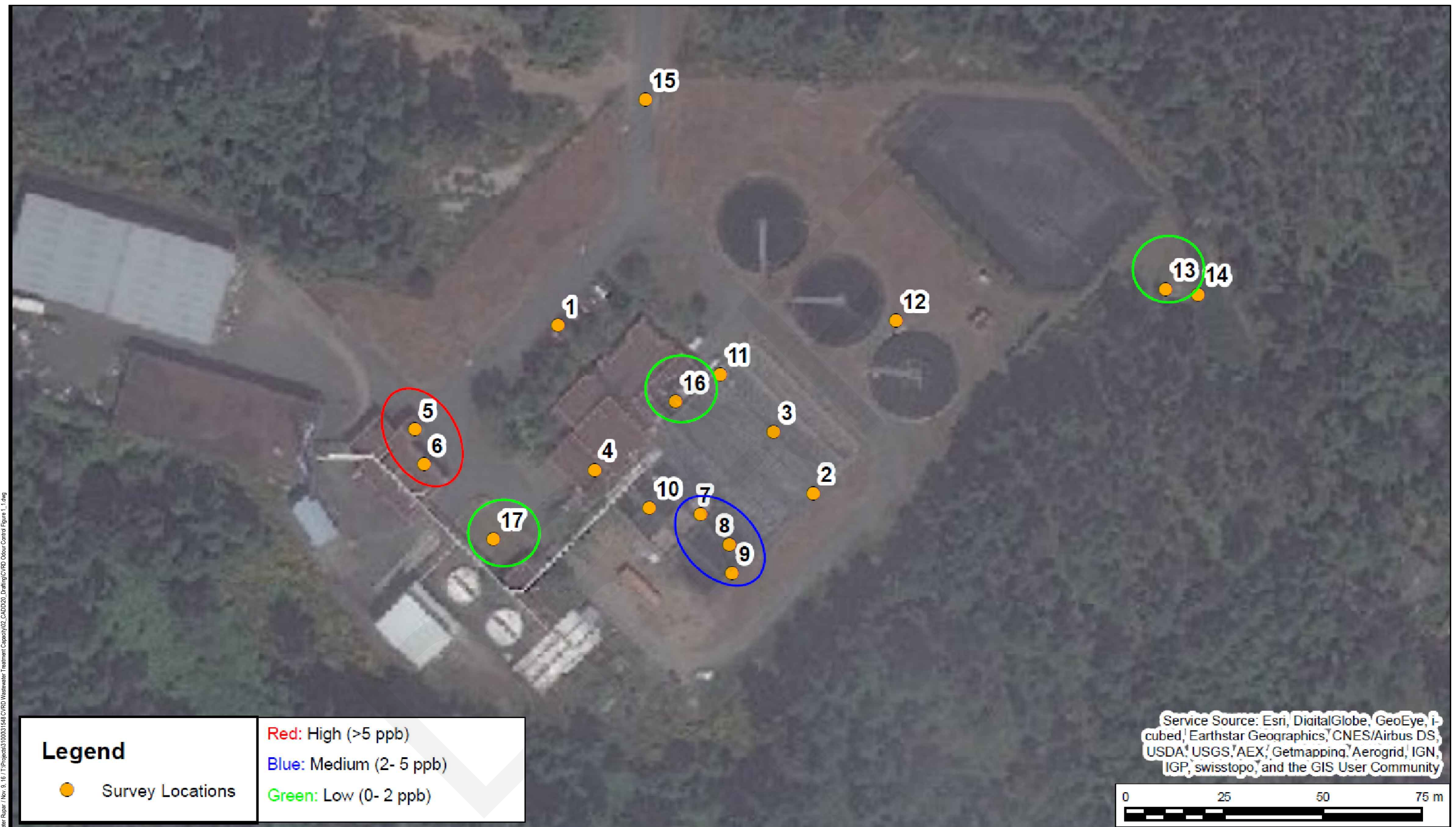
CVWPCC - ODOUR CONTROL OPTIONS HYDROGEN SULFIDE SAMPLING LOCATIONS IMAGE ADAPTED FROM RWDI (2015)
