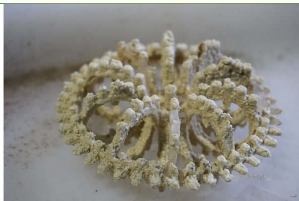
Existing Scrubber Media: Jaeger Tripack with solid deposits.
